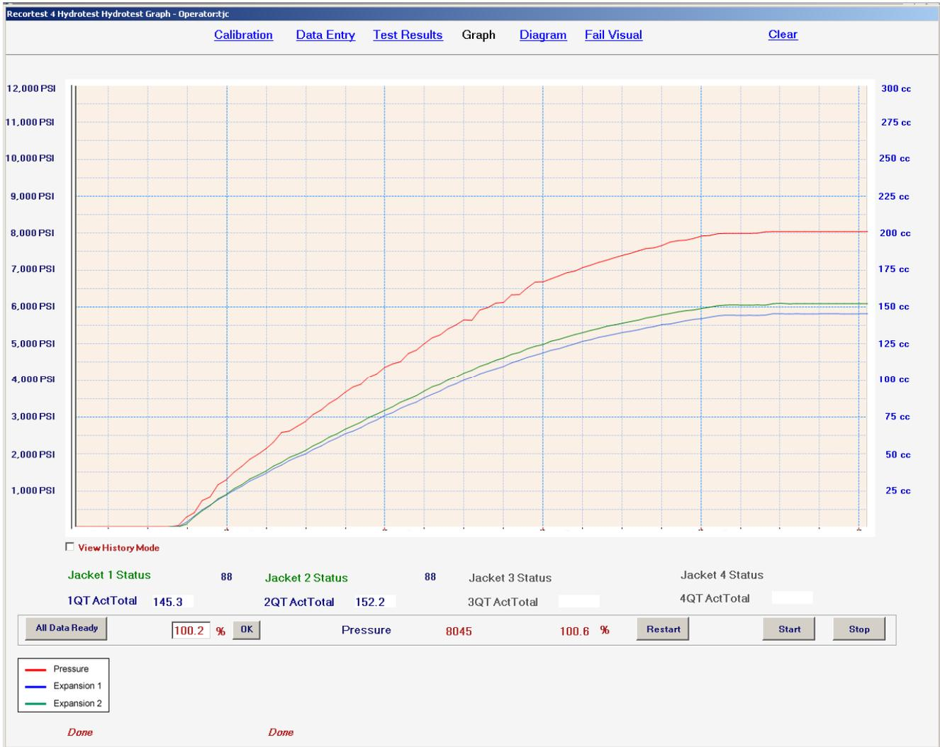
Shown above are the graphed curves of the pressure, and cylinder expansions. 2 cylinders are shown to be pressurizing at the same time. The scale of the graph can be changed for different viewing if needed.
