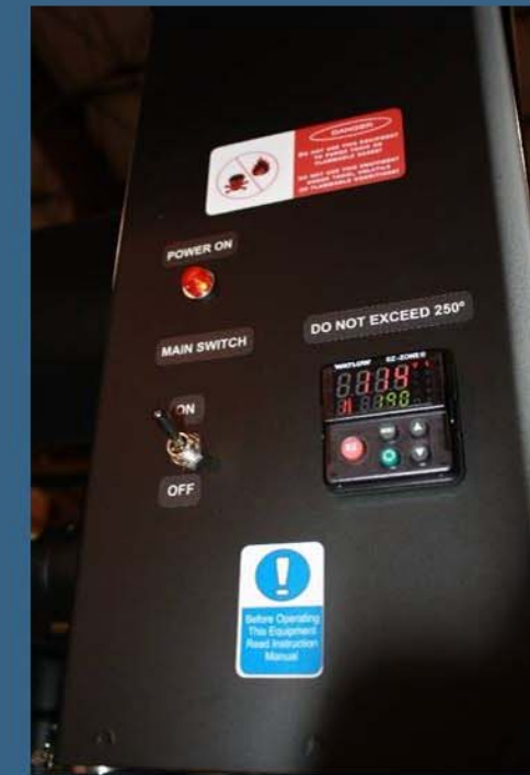
Digital Controller with Temperature Readout *Optional Separate Display With Temperature Thermocouple
